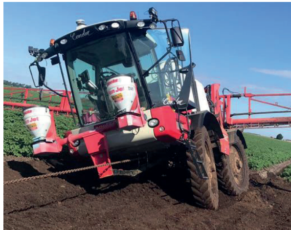
Pictures above and following illustrate further UK farm examples of this version of the sprayer becoming bogged in break crop, and root crop fields respectively. Pictures c/o Jack Smith, AG Wright & Son Hillrow Causeway, Ely, Cambs.
