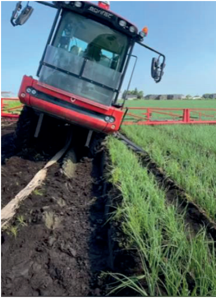
Pictures above and following illustrate further UK farm examples of this version of the sprayer becoming bogged in break crop, and root crop fields respectively. Pictures c/o Jack Smith, AG Wright & Son Hillrow Causeway, Ely, Cambs.
