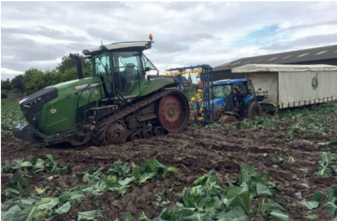
[Above: TH Clements vegetable harvester & tractor being towed out of ruts. The tractor has sunk to >1m as shown by the measurement (inset) of the front wheel. This is shown approximately to scale in the picture following]
