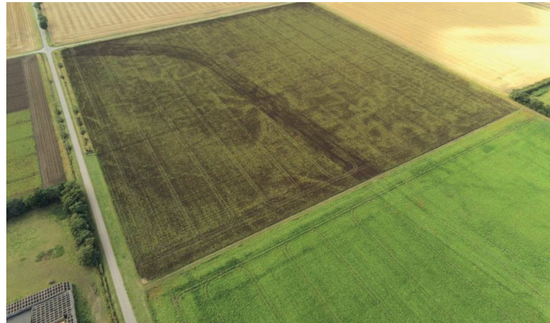
Below: Triton Knoll cable effect near Sibsey Northlands in two crops showing different growth stages and resulting inconsistent crop canopy effects. These are crops coming to the second, and third harvests since reinstatement respectively.
