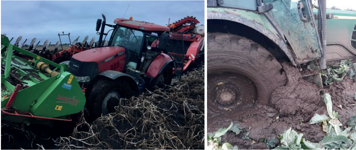
[Above, & below: examples of potato and vegetable harvesting equipment becoming bogged down, otherwise known as “falling through” soils]
