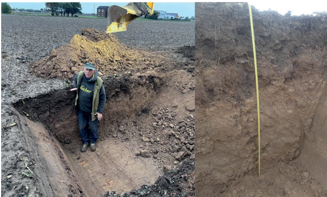
[Above: profile showing 3 distinct layers, 0 to 0.4m, 0.4m to 0.7m, with the subsoil below]
