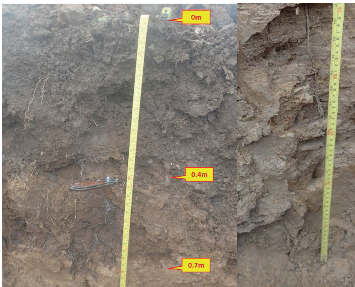
[Above, left: knife position at the 0.4m depth. This has darker, higher organic matter content fine silt loam above, and lighter, reduced organic matter content, slightly coarser silt loam below to 0.7m. These layers provide a balance of water and nutrient to the crops. Both layers clearly have high volumes of roots from the last crop harvested. Right: below 0.7m,, the sandy silt loam subsoil also has roots passing through, these are reduced in volume, and provide the crop with access to water mainly]
